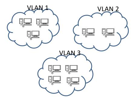
The diagram above represents VLAN segments where only the users or nodes in VLAN 1 can communicate with each other. This segmentation provides security as well as traffic optimization.
