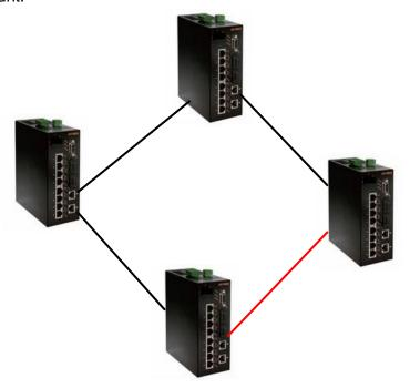
In the diagram above the red link is set to standby mode and will not transit packets unless a break or failure occurs in one of the other links. This represents the basic spanning tree operation where link redundancy is achieved without creating data loops.
