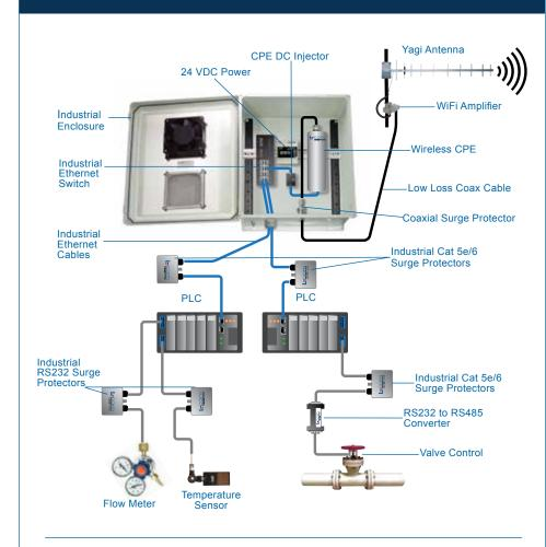
This diagram encompasses a rugged indoor NEMA enclosure, along with Ethernet, RS232, RS485 and WiFi connectivity, to provide an end-to-end process automation networking solution.
