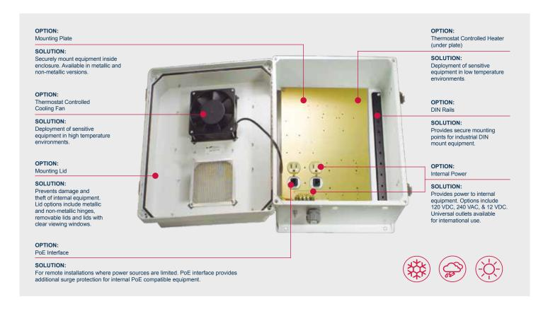
L-com offers one of the most extensive lines of NEMA rated enclosures in the industry. These enclosures can be used for wired, wireless and industrial networking applications, both indoors and outdoors and come with many options for heating, cooling, venting, and internal power requirements.
