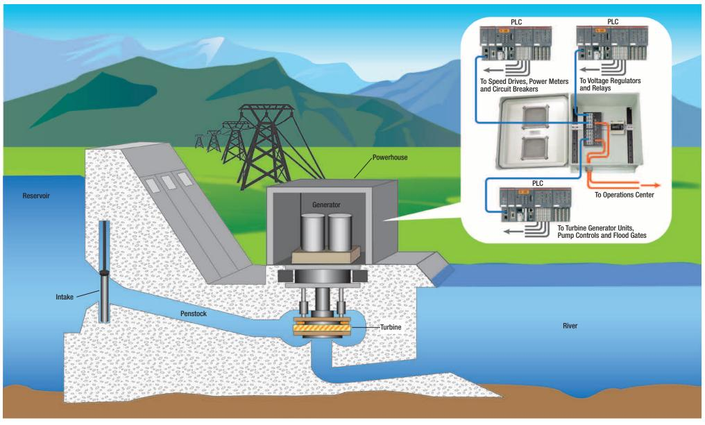
This diagram depicts a hydroelectric dam control network which utilizes L-com's industrial NEMA enclosure, IES series industrial Ethernet switch, fiber optic cables and our industrial grade Ethernet cables to provide monitoring and control of the hydroelectric dam turbine, flood gates and other critical systems.
