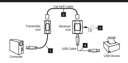
Connect source and transmitter unit with USB A-type pigtail cable
