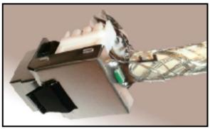
3. Pierce bayonet between braid and aluminum foil all the way down and hit the shoulder. Place the cable tie-holder over the braid as photo illustrates.
