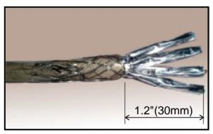
2. Bend back the copper braid over sheath.
