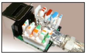
After termination completed, make sure the aluminum foil fully covers the wires all the way down to the punch block.
