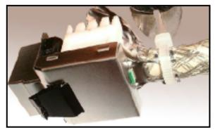
4. Place cable tie at assigned place. Squeeze the cable tie and cut the cable tie tail.
