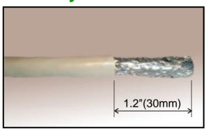
1. Strip the outer plastic jacket with appropriate length about 1.2 inches (30mm)
