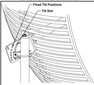
To mount antenna assembly in a tilted position, attach (1) U-Bolt assembly to either the fixed tilt positions or to the tilt slot (as shown) on the "L" Bracket.
