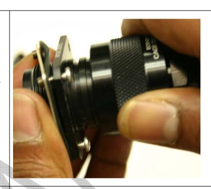
Screw the Rear Extension Cap onto the Main Connector Housing and tighten with a 9/16" wrench.
