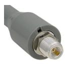
The HGV-4959 Series antennas feature an integral N-Female bulkhead type connector that can mount through the wall of an equipment enclosure. Also included is a mast mounting kit which consists of a heavy-duty steel bracket and a pair of Ubolts. This kit allows installation on masts up to 2.0" in diameter.
