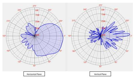
2300-2700 MHz / 5150- 5850 MHz, 17 / 20 dBi, Wifi MIMO Sector Antenna, 65-degree, +/-45 Dual Pol, 2-Port, Type N Female
