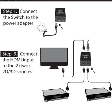
Step 2. Connect the HDMI output to display
