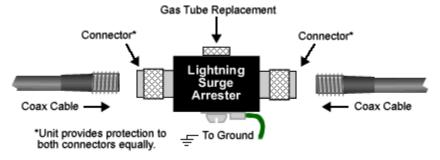
Operational Note: This 1/4 wave protector is not for use with coaxial cables carrying a DC voltage such as in the case of a remote-mounted amplifier or LNA. For applications requiring DC capability please see our Gas Tube version AL-NMNFB-9.
