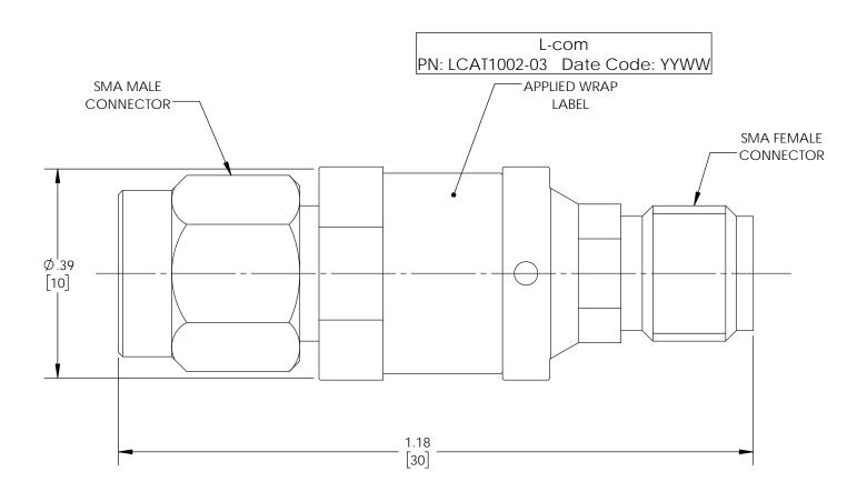
UNLESS OTHERWISE SPECIFIED LEADING DIMENSIONS ARE INCHES DIMENSIONS IN [] ARE MILLIMETERS TOLERANCES: .X=± .2 [5.08] FRACTIONS .XX=± .01 [.25] ± 1/32 XXX=± .005 [ .13 ] ANGLES ± 1°
