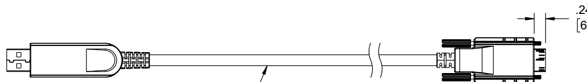
USB 3.0 HIGH FLEX CABLE JACKET: PVC, BLACK NOM DIA.: .217" [5.5]
