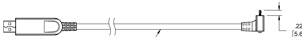
USB 3.0 HIGH FLEX CABLE JACKET: PVC, BLACK NOM DIA.: .217" [5.5]
